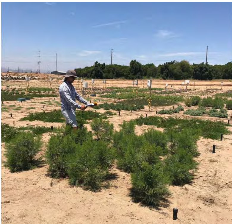
Ph.D. student Anish Sapkota collecting NDVI data using a handheld sensor.
