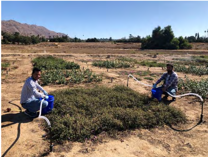
Ph.D. students Anish Sapkota and Amninder Singh calibrating the flowmeters for accurate measurement of applied water.
