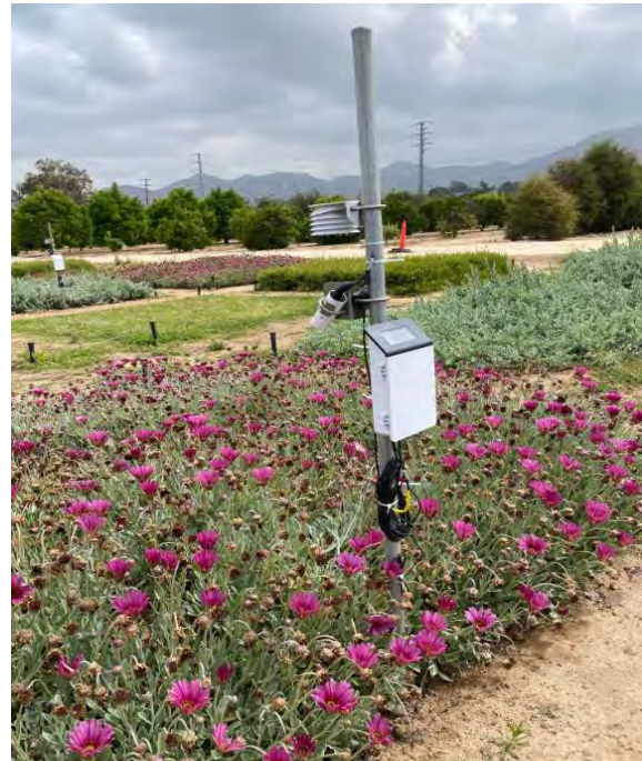
Fig. 3. Weathermatic ET-based smart irrigation controller (left) and infrared radiometer for canopy temperature measurement (right)
