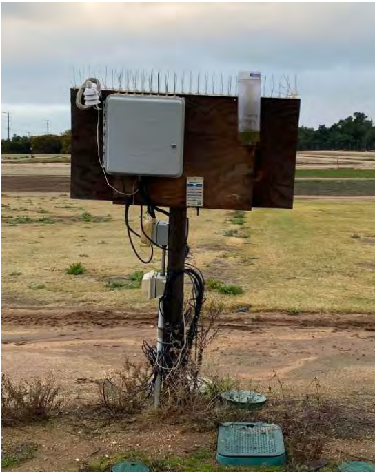
Fig. 3. Weathermatic ET-based smart irrigation controller (left) and infrared radiometer for canopy temperature measurement (right)
