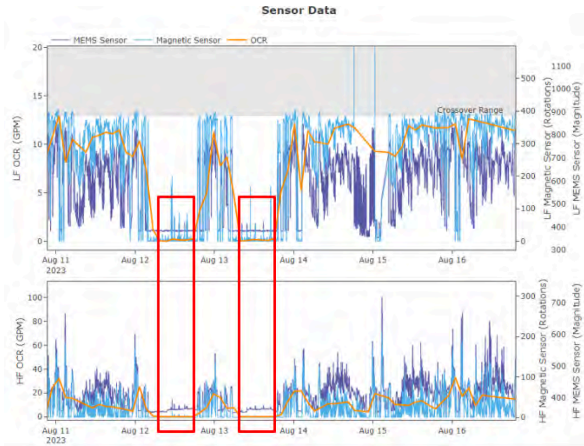
Figure 15 - Meter experiencing an early crossover valve error
