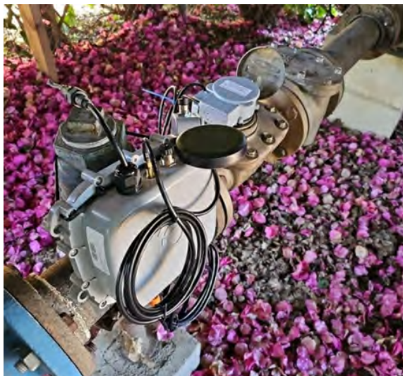
Figure 2 - Edge computer connected to the sensors, with the cellular antenna.
