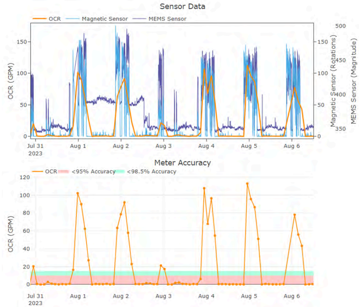
Figure 27 - Meter experiencing an oversized meter error condition
