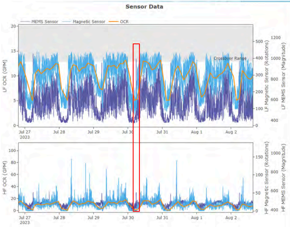
Figure 16 - Meter experiencing an early crossover valve error
