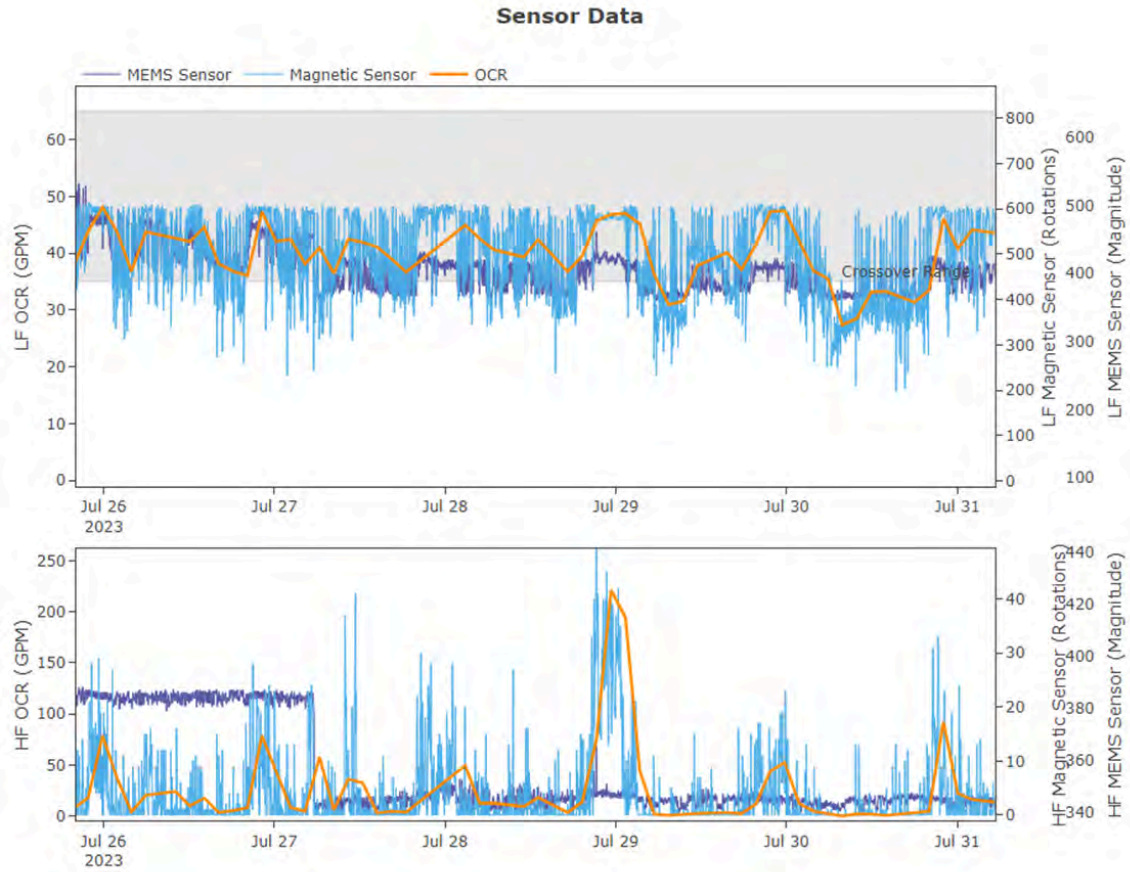
Figure 18 - Meter experiencing a damaged register
