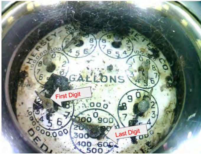
Figure 21 - Damaged register & incorrect meter configuration
