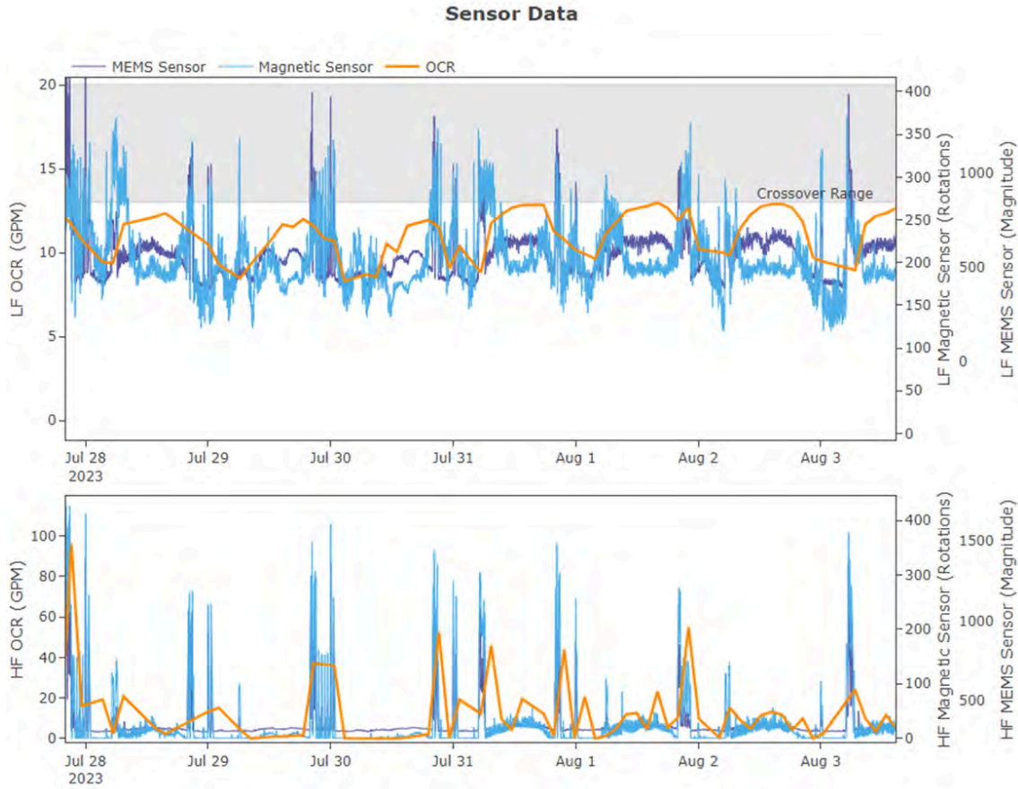
Figure 22 - Meter experiencing a damaged register
