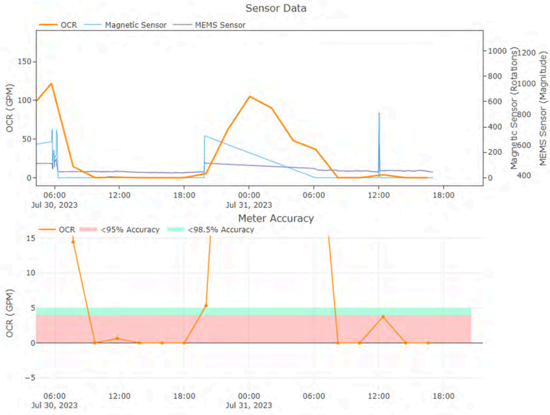
Figure 32 - Zoom showing flow outside of meter operating range
