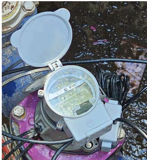
Figure 1 - Camera and sensor pack containing the hall effect and acoustic sensors.
