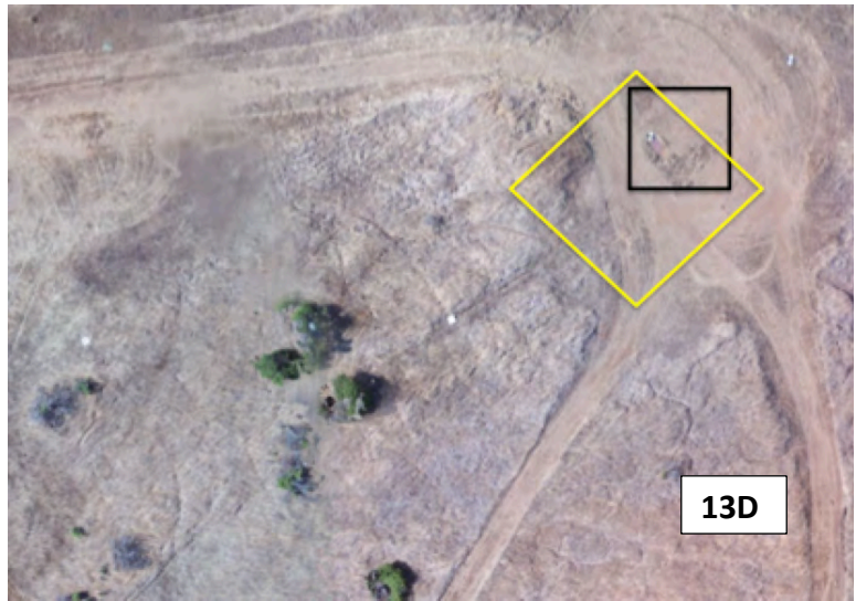
Figure 13A, B, C, D. Figure 13A. Visual (P4P) and Figure B reflectance (M200) aerial maps illustrate the MPWD1 site. The green areas in Figure 13B reflect cooler temperatures, while the yellow-orange areas reflect warmer temperatures. Figure 13 C shows the reference location for the enlarged view in Figure 13D. The square on Figures 13A, 13B, and 13D outlines the general area of the valve box (approximately 4.5 ft. subsurface) – the location of the simulated ‘leak’; the diamond shows the general area with lower temperatures. This area is interpreted as: ‘affected by the simulated leak’ – with temperatures approximately 10F lower than the surrounding ground on the dirt road. By comparison, the ovals (13A, 13B) to the left show how vegetation appears as a temperature anomaly, an artifact on the reflectance map.
