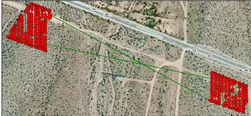
Figure 19A. Aerial mapping using sUAS DJI M200 XT2 and DJI Pilot software for LVVWA2, sections 2.1A-B and 2.2A-B. The red dots represent the flight path and images taken during flight. (Source: MW, 2019).
