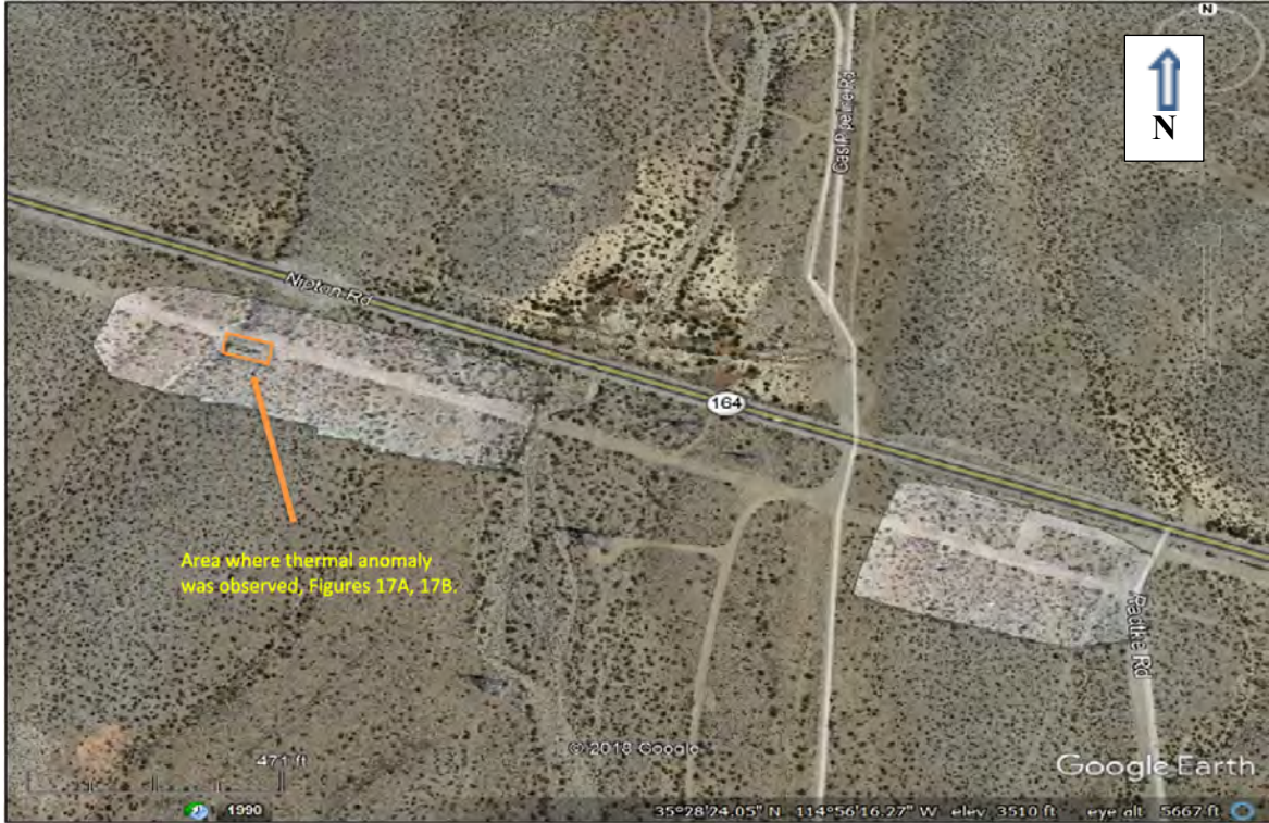
17B. Aerial orthomosaic map, generated using DJI Phantom 4 Pro and Pix4D Mapper software, for LVVWA S2-1AB, S2-2AB. (Source: MW drone flight, 2019). The water pipeline runs parallel to the south side of the dirt road. Note: orange box shows the location of a thermal anomaly observed on May 27, 2019.
