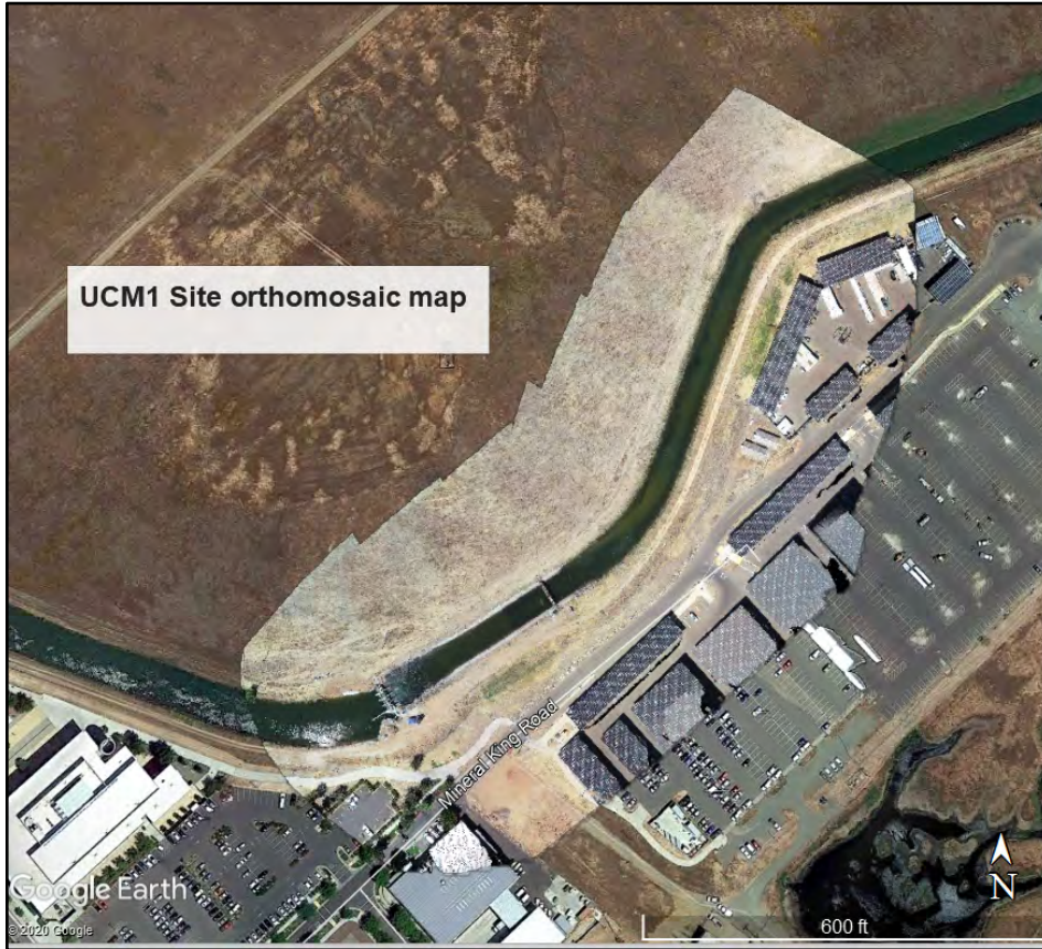
Figure 8. Orthomosaic map of UCM1 field site, generated using DJI P4P drone and Pix4D image Capture and Mapper processing software (lighter area). Surrounding area image uses Google Earth satellite view. Note the much higher resolution of the drone image, since it has a ground sampling distance (GSD) of approximately 1 inch and the satellite view has a nominal GSD of 50 feet.
