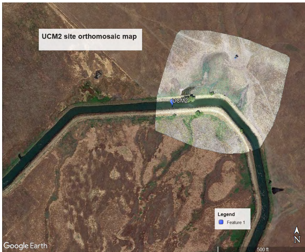
Figure 10. Map of UCM2 field site, generated using DJI P4P drone and Pix4D image Capture and Mapper processing software (lighter area). Surrounding area image uses Google Earth satellite view. Note the much higher resolution of the drone image, since it has a ground sampling distance (GSD) of approximately 1 inch and the satellite view has a nominal GSD of 50 feet.
