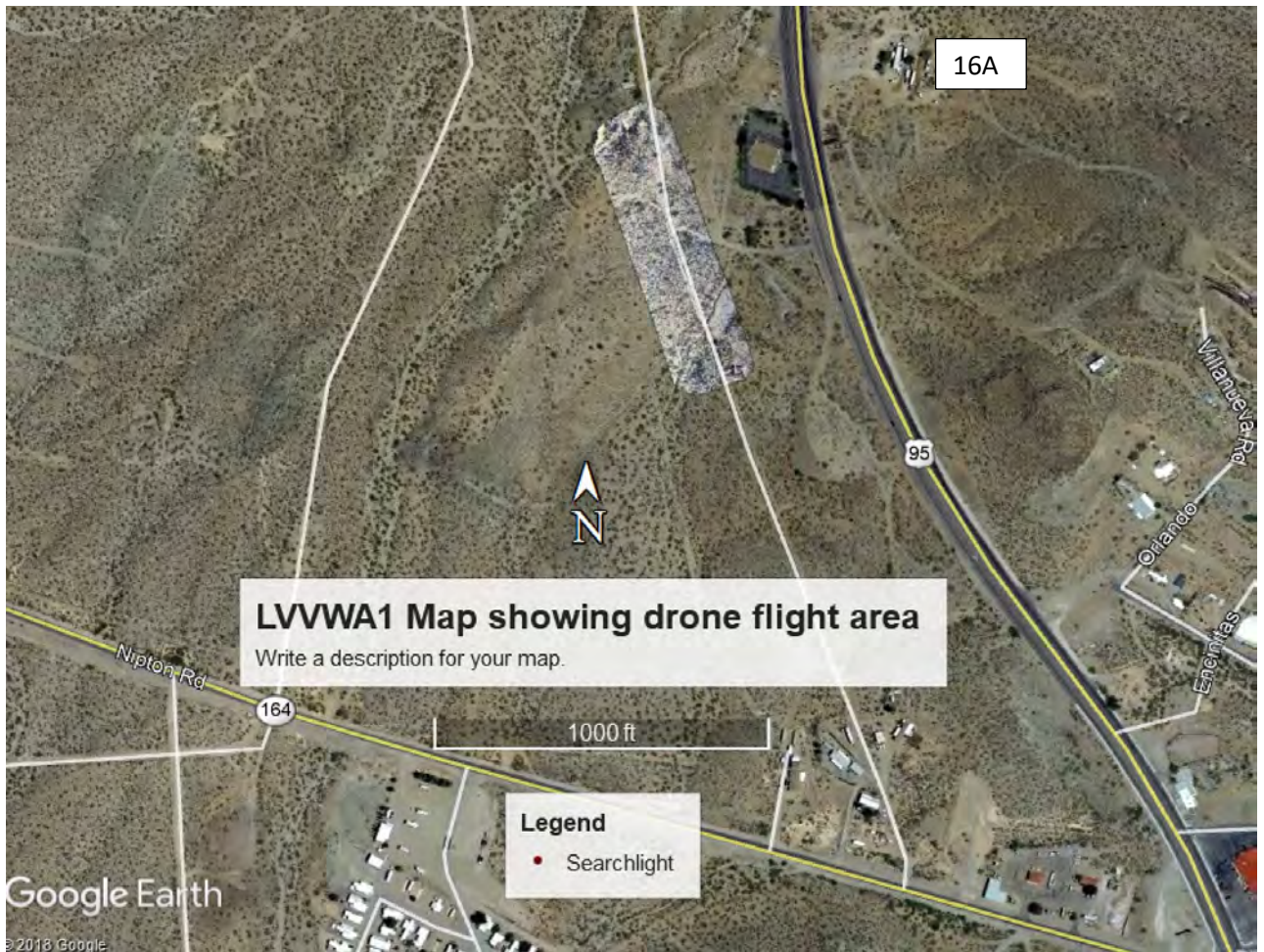
Figure 16A. Flight map (lighter area), using sUAS DJI P4P and Pix4D Capture for LVVWA1.
