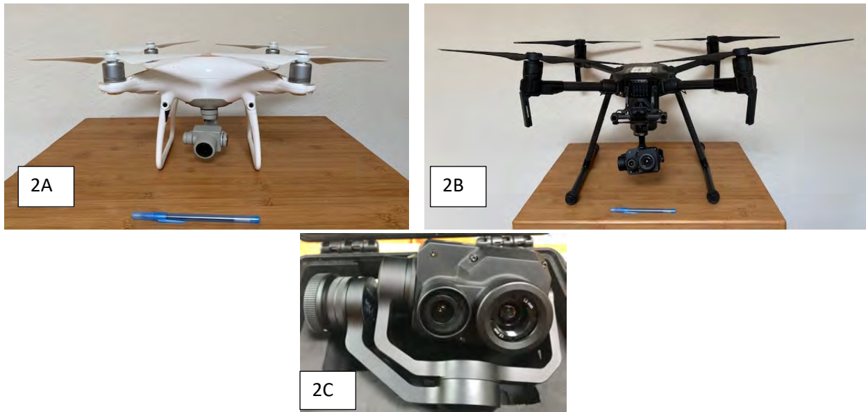
Figure 2A. DJI Phantom 4Pro with its 20-MP, high resolution visible light (RGB sensor) camera (pen for scale), Figure 2B. DJI Matrice 200 with ZenMuse XT2 dual lens camera (visible light, 12-MP, RGB sensor and 13mm thermal sensor), and Figure 2C, close-up view of the XT2: visual (left) and thermal (right). The XT2 captures
