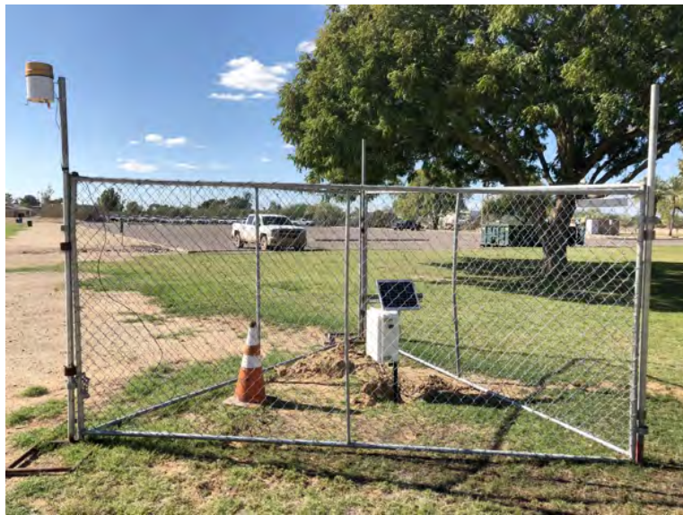
Figure 4. Study site location at Paradise Valley Park (top) with control and treatment plots. Photograph of the x1 station with fence (bottom), which includes a solar panel, rain gauge, and soil moisture sensors.
