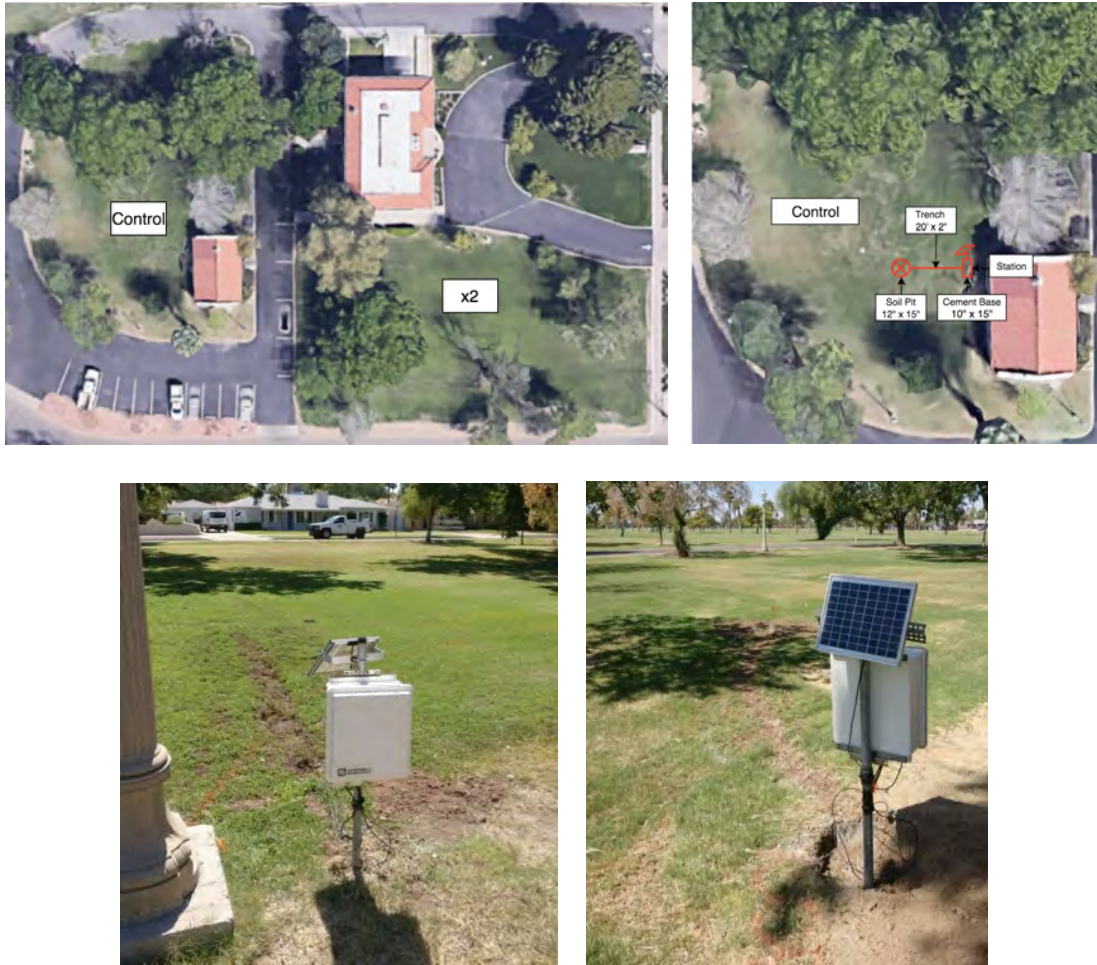
Figure 3. Study site locations at Encanto Park (top) with control and x2 treatment plots. Soil moisture stations installed (bottom) at the x2 treatment (left) and control plot (right).
