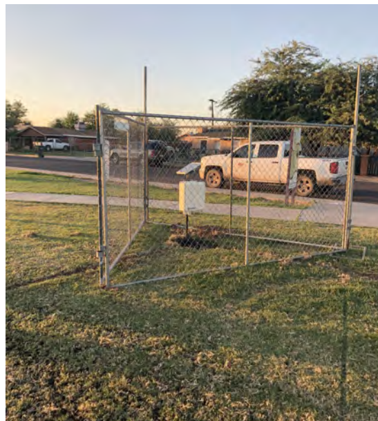
Figure 5. Study site location at Smith Park (top) with control and treatment plots. Photograph of fenced soil moisture station (bottom), which includes a solar panel, datalogger, rain gauge, and soil moisture sensors at multiple depths.
