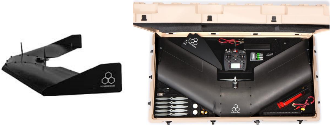
Figure 1. The Honeycomb AgDrone™ fixed wing agricultural Unmanned Aerial System (UAS) used for aerial data capture for project ICP 167775. (Source: Honeycomb Corp.)
