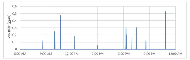
Table 3 summarizes the results. Ultimately, the i.ScoopShower used 0.28 gallons per use. If 17.7 uses per day are applied to the baseline dipper well, the dipper well would be consuming 27 gallons per use and 100 Wh per use in embedded energy. Anecdotal evidence was collected by a brief interview with staff at the site. Staff adapted quickly and easily to using the new device, and no major operating problems or staff frustrations were reported.
