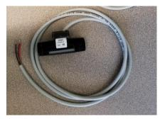
Power metering was accomplished with a Continental Control Systems Watthode Pulse electricity meter and current transformers. This combination had accuracy  $\pm 1\%$  for current between 1 and 50 A (Figure 6).
