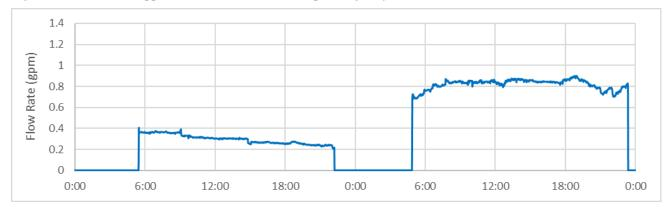
Figure 10. Los Banos Dipper Well June 13<sup>th</sup> and 14<sup>th</sup> Operating Profile
