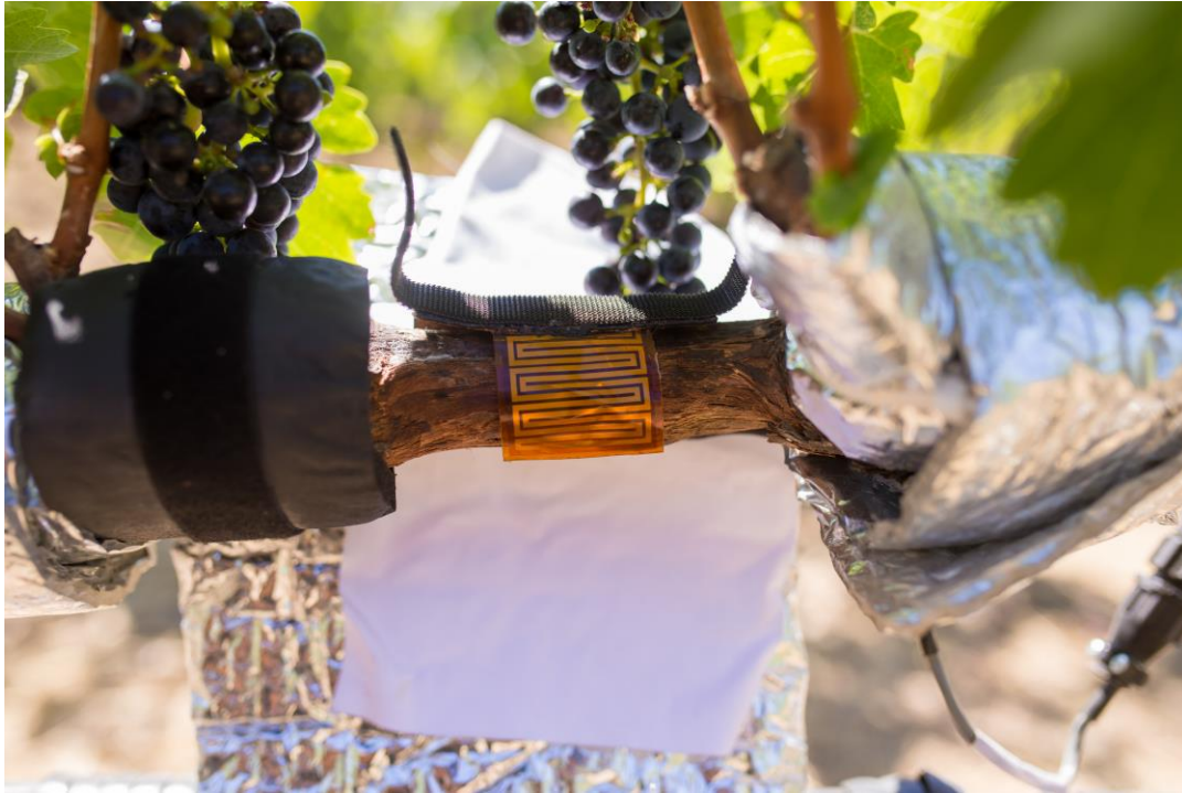
FIGURE 7: SAP FLOW SENSOR AND STEM SECTION. THE SENSOR IS WRAPPED AROUND THE STEM TO MONITOR VINE SAP FLOW.
