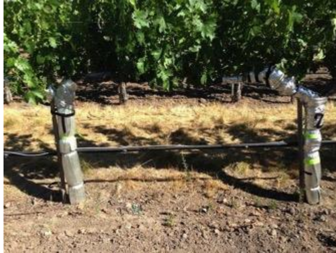
FIGURE 8: TWO VINES EQUIPPED WITH SAP FLOW SENSORS AND INSULATED.
