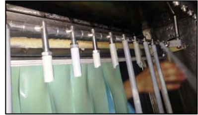
Figure 70: Broken rinse sensor fingers
