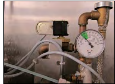
Figure 37: Rinse pressure gauge reading at 17.5 psi
