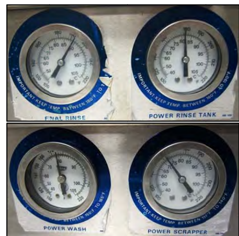
Figure 50: Temperature gauge readings on dishwasher during rinse operation
