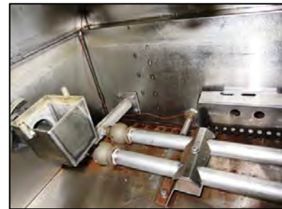
Figure 87: Instrumentation box and ultrasonic water meter transducers
