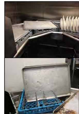
Figure 29: Conventional washing of sheet pans (top) vs. efficient washing of sheet pans (bottom)
