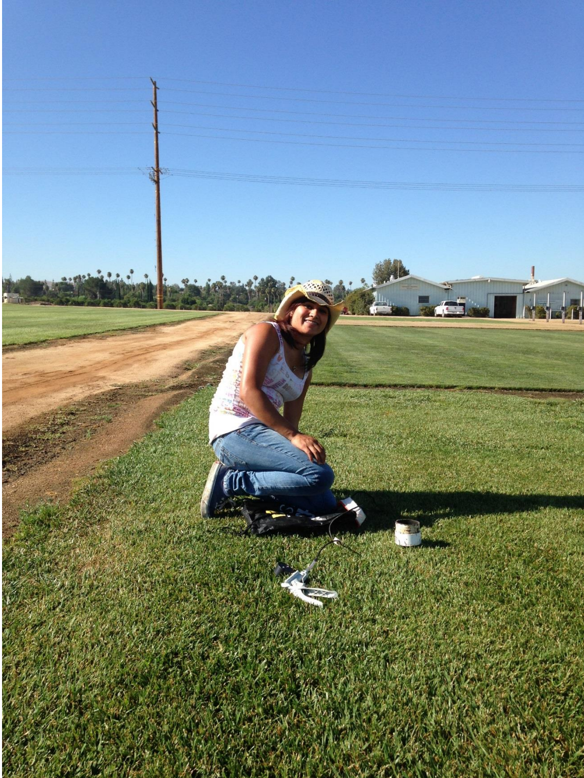
Undergraduate Jacky Corona extracting water from lysimeters in turf plots at UCR to determine biochar's effect on fertilizer efficiency. Jacky
