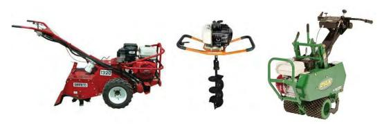
Figure 5. Photographs of larger rain garden installation equipment: tiller (left), auger (center), and sodcutter (right). Images courtesy asrentall.com and HomeDepot.com.
