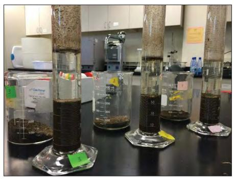
Figure 14. Lab measurement of soil texture from individual rain garden sites.
