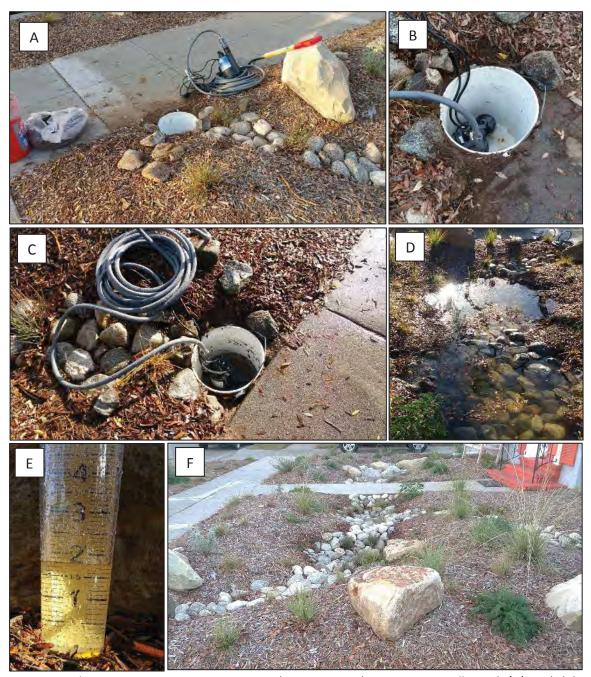
Figure 17. Post-implementation stormwater monitoring (Site 2, Wagner). Pre-storm installation (1/4/2016): (A) 5-gallon bucket installed at bioswale overflow; (B) automated pump, hose, and water meter to assess installed. Post-storm assessment: (C) Bioswale overflow monitoring post-storm (1/5/2016); (D) bioswale ponding (1/5/2016); (E) on-site rain gauge (1/5/2016); (F) complete bioswale infiltration (1/6/2016).
