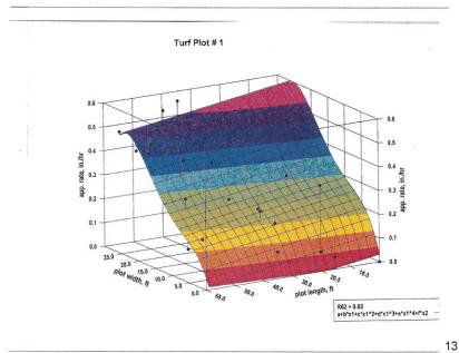
Computer Generated Model of Irrigation Distribution (Red = Area of Lightest/Pink Area of Heaviest Application of Water)
