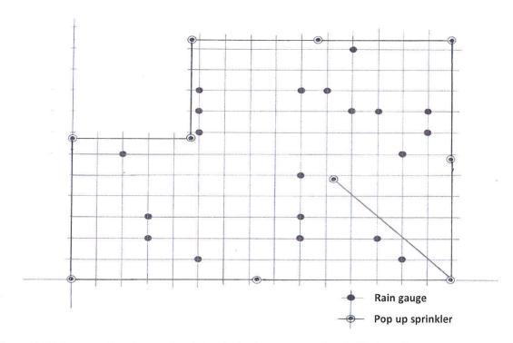
Figure 1. Hydrozone showing randomly located rain gauges and sprinkler locations. (Note: Grid spacing, 2 ft X 2 ft)
