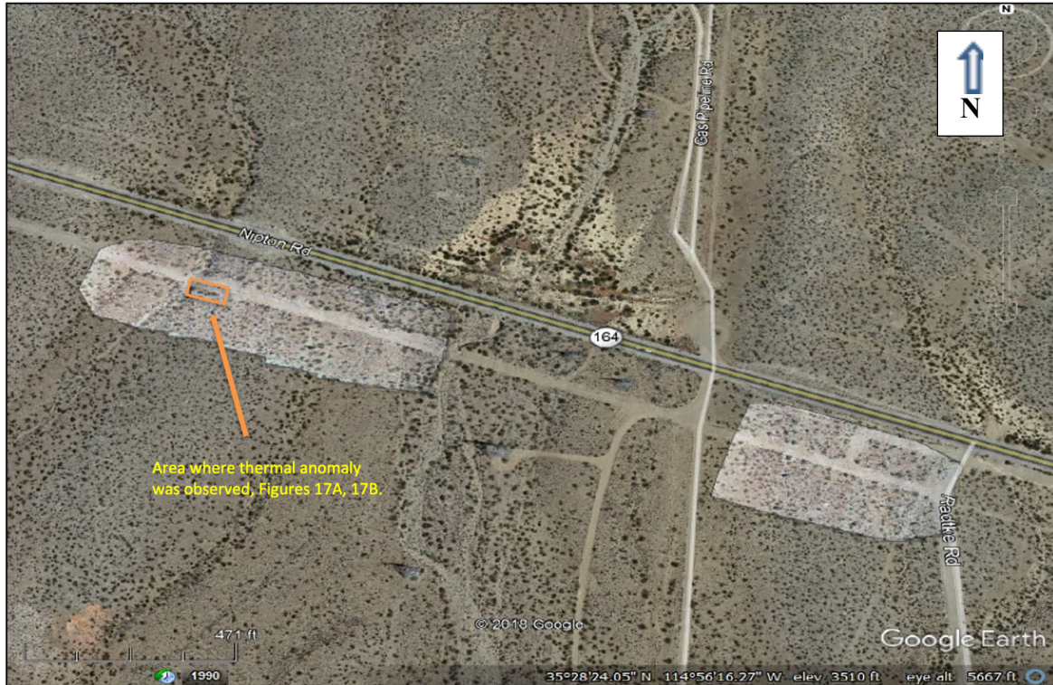
17B. Aerial orthomosaic map, generated using DJI Phantom 4 Pro and Pix4D Mapper software, for LVVWA S2-1AB, S2-2AB. (Source: MW drone flight, 2019). The water pipeline runs parallel to the south side of the dirt road. Note: orange box shows the location of a thermal anomaly observed on May 27, 2019.
