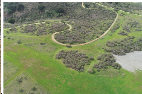
Figure 12B. Aerial views of MPWD1 site on March 19, 2019, with abundant grassy area due to recent and prolonged rainy season. The ground temperatures were too low due to the cooling effect of the green vegetation, resulting in insufficient contrast between the ground surface and water temperatures. The lack of contrasting ground to water temperatures resulted in no discernible temperature anomalies. Figure 12C. shows the aerial orthomosaic map for the MPWD1 site on July 26, 2019, almost two months after last rain event, with grassy areas dried out and ground temperatures (>100F) more than 40F higher than the water (60F). The orthomosaic map was developed using the P4P drone and Pix4D Capture and Mapper software.
