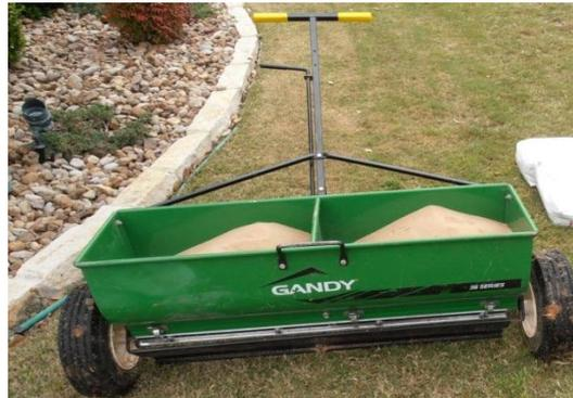
We used two different application rates of AquaSmart PRO. The product is available in 40 lb. bags so we applied 20 lbs. per 1000 sq. ft. on two yards and 40 lbs. per 1000 sq. ft. on the other two yards. Once the product is applied it is recommended to give it a solid watering to activate the product.
